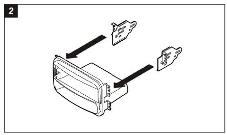
Snap the ISO Brackets over the mounting tabs on the Radio Housing.
